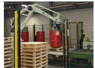
Kawasaki CP500L at Shell (B) 200L vaten palletiseren
